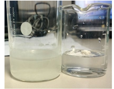
Dispersibility of PEEK-powder in water: plasma-treated powder (left), untreated powder (right)
