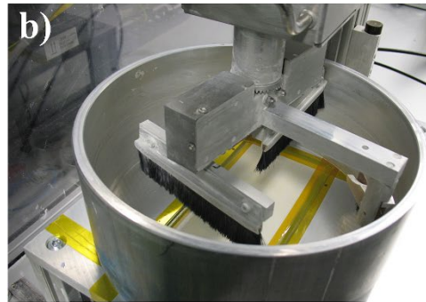
a): Schematic view of the powder treatment reactor, b): photography of the reactor
