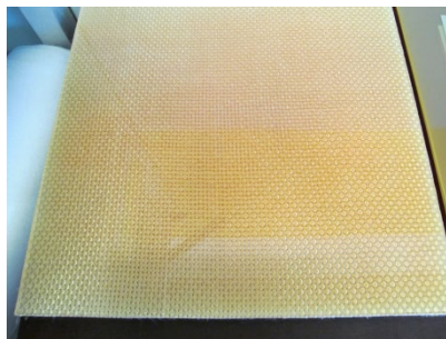
Powder-coated glass pane with integrated glass fibre fabric
