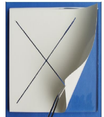
Powder-coated glass panes using the developed surface activation
