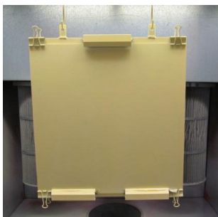
Vertical coating of glass surfaces with powder coating
