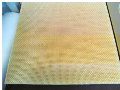
Powder-coated glass pane with integrated glass fibre fabric
