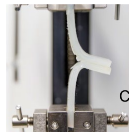
A - tensile shear test; B - bend test; C - peel test; D - punch break test; E - test specimen for punch break
