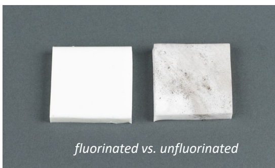
Comparison of soiling tendency of fluorinated and untreated silicone surfaces
