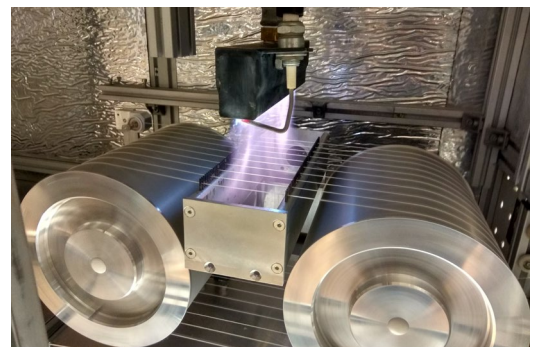
Yarn treatment using flame treatment
