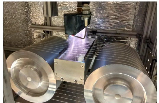
Yarn treatment using flame treatment
