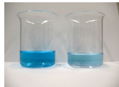
Methylene blue solution before (left) and after 3h UV irradiation (right)
