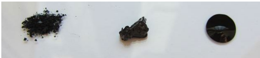
Adjustable texture of nanoparticle - oleic acid - dispersion by tuning the particle-concentration (left: powder with 90% NP, middle: paste with 50% NP, right: oil with 25% NP).
