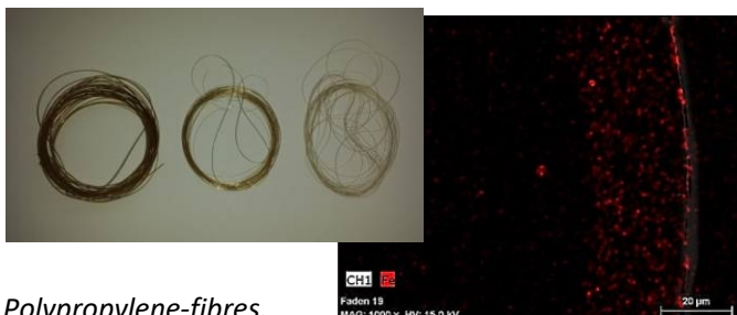
Polypropylene-fibres, surface modified using core-shell nanoparticles (left). Increased concentration of particles on the fibre surface after treatment in a magnetic field (EDX-picture)
