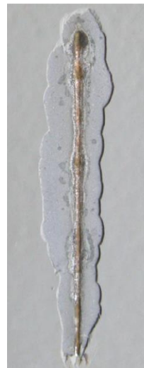
standard evaluation of corrosion, delamination
