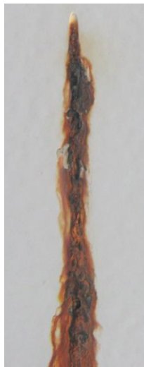
epoxy coating 800 h SST
